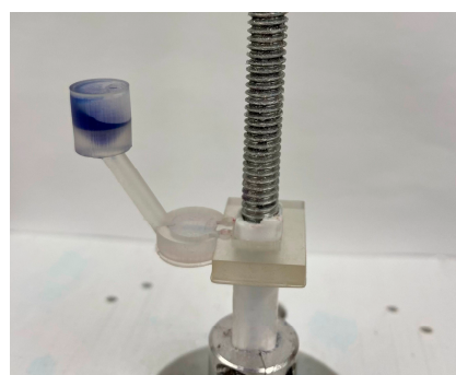
Figure 15. The gravity mixer with a 700 \mu\text{m} diameter slope channel after mixing.
