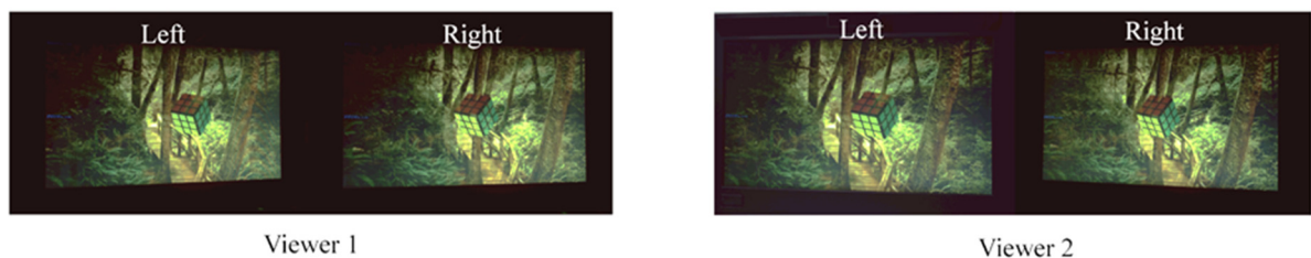
Figure 9. The display performance for dual viewers at a viewing distance of 750 mm. The left and right eyes' visual perception show a significant disparity, which can be seen by the relative position of the tree and the small rhomboidal grid.
