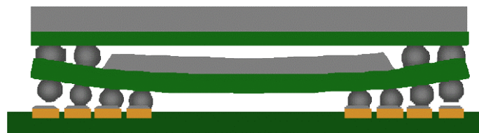
Figure 3. Open joints due to warpage of Package on Package (PoP) [11].
