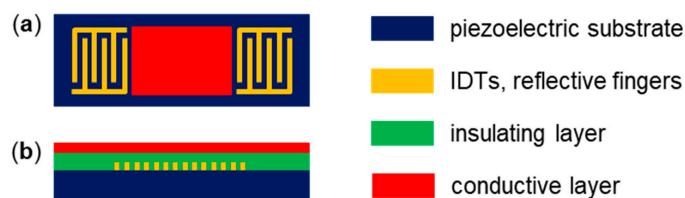
Figure 2. Introduction of electrically shielding layers on SAW sensor devices. (a) Conductive layer in between the IDTs of a delay line device (top view). (b) Conductive layer with insulating intermediate layer on a one-port resonator (side view).
