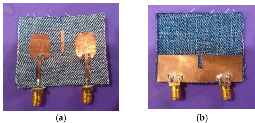
Figure 5. Proposed textile irregular octagon antenna. (a) Top view. (b) Bottom View.
