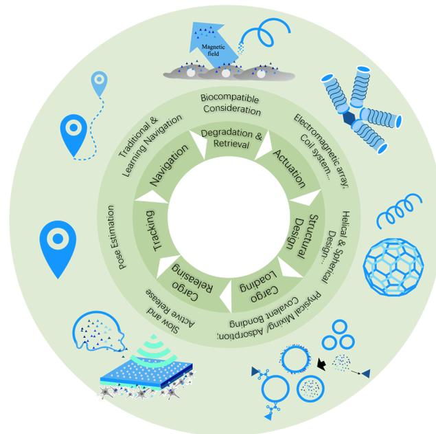
**Figure 1.** The concept figure of this review. We systematically decouple recent works on MMRs for in vivo cargo delivery into a structured framework. The framework includes magnetic field actuation, structural design, cargo loading and release mechanisms, tracking, navigation, as well as the degradation and retrieval of MMRs.
