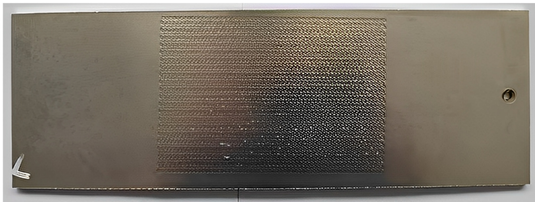
Figure 11. Aluminum alloy plate forming effect under laser energy 7 J.
