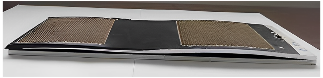
Figure 5. Results of laser peening molding of S-shaped parts.
