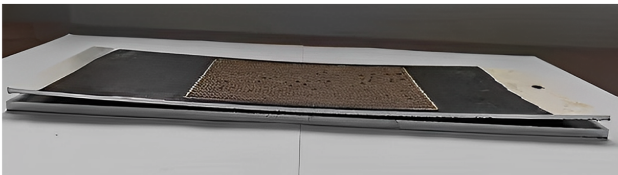
Figure 13. Effect of laser peening forming of aluminum alloy plate with a thickness of 2 mm.
