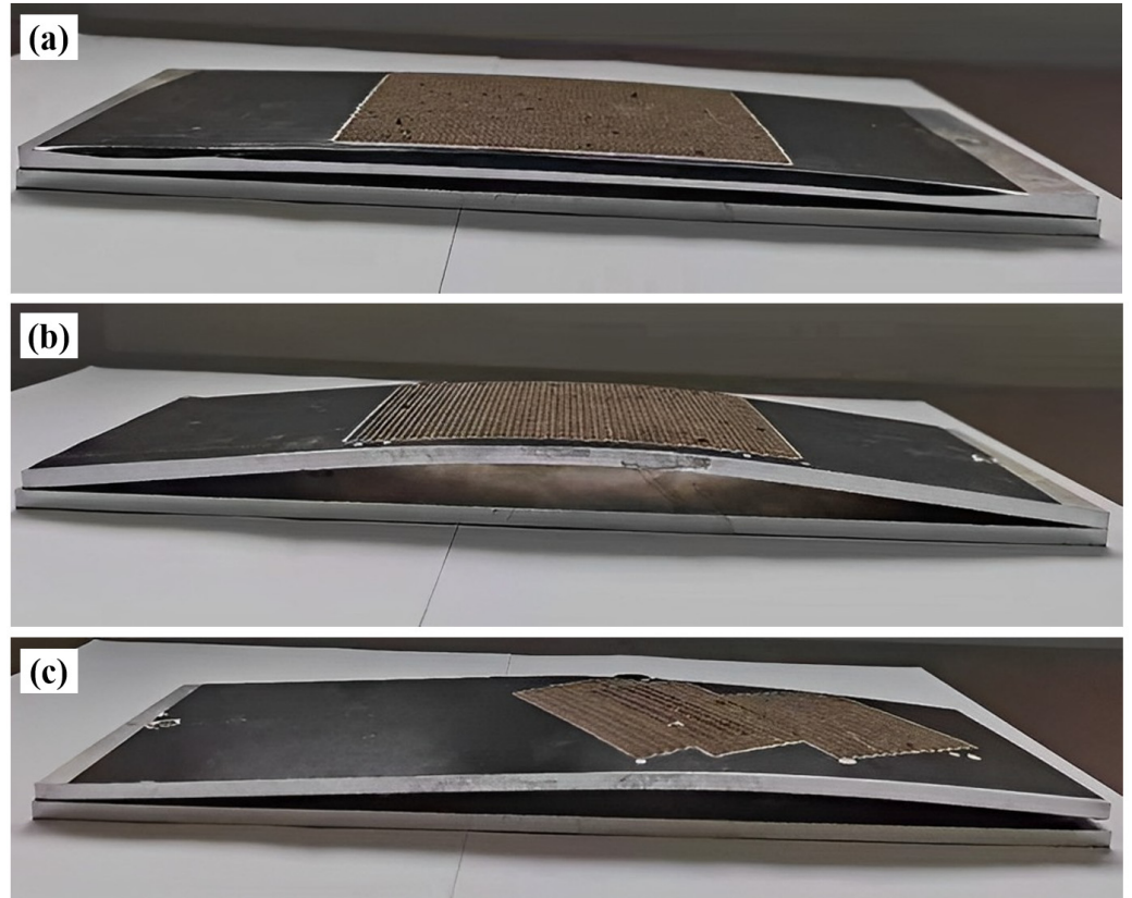
Figure 7. Effect of different laser peening paths on plate forming: (a) Impact path 1; (b) Impact path 2; (c) Impact path 3.
