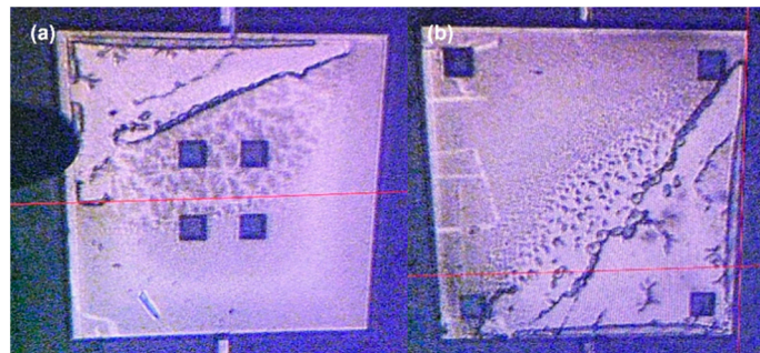
Figure 12. The black substance on the metal layer after secondary anodic bonding. (a) Structure with 4 windows in the center (b) Structure with 4 windows around the edges
