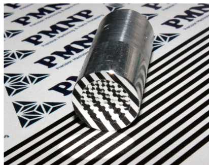
Figure 5. Photograph of a hexagonal microlens array on aluminum alloy machined by segment STS turning at N = 45 rpm.
