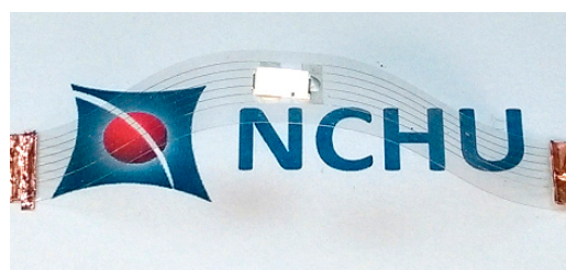
Figure 8. Demonstration of conductive silver line fabricated by LDSP on the transparent PET substrate.
