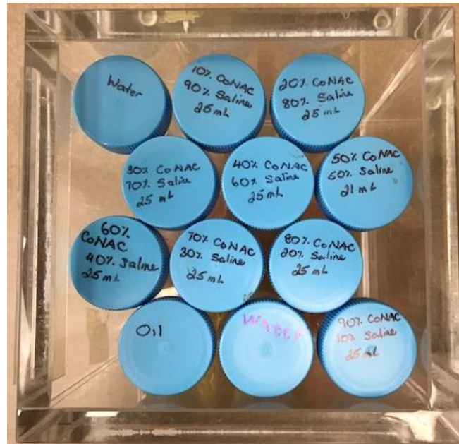
Figure 1. Test solutions for magnetic resonance imaging (MRI). Each of the C4/saline (C4:S) solutions, with C4:S concentrations varying from 10%:90% to 90%:10%, were placed in nine 50 mL polypropylene centrifuge tubes. Three additional tubes, two filled only with water and the other filled only with oil, were used as controls. The 12 tubes were placed as shown in an acrylic box, which was filled with water and placed at the center of the MRI scanning field.
