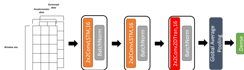
Figure 10. Two-channel ConvLSTM architecture.
