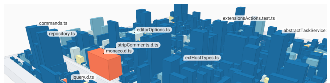
Figure 1. A 2.5D interactive software map visualization of the Microsoft vscode software project. The number of lines of code (LoC) is mapped to weight, the number of functions (NoF) is mapped to height, and the density of comments (DoC) is mapped to color, ranging from inconspicuous (blue) to conspicuous (red).
