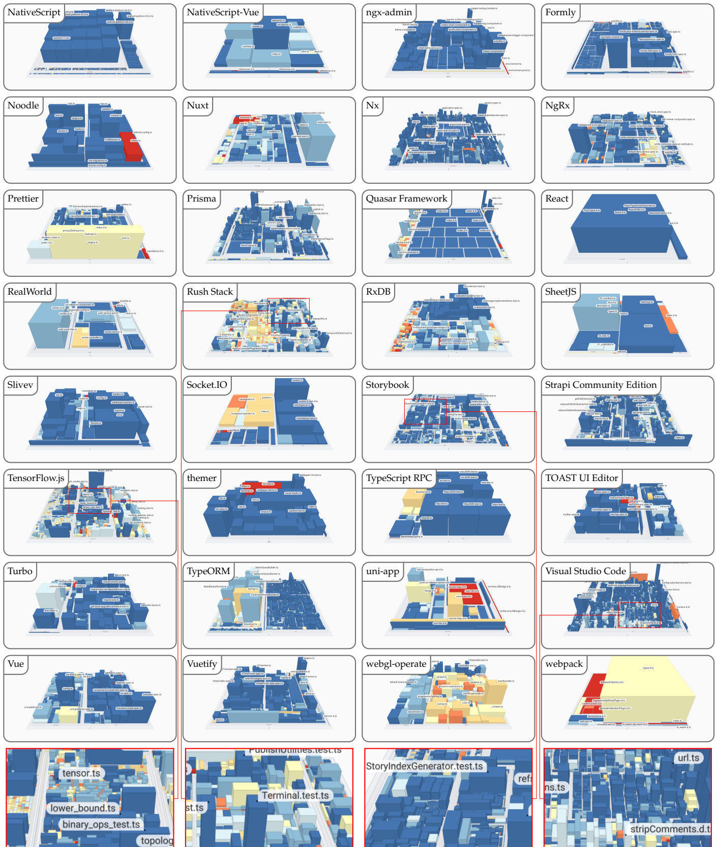
Figure A2. Comparison of the second half of of TypeScript projects with increasing size and complexity using a software map visualization. The number of lines of code (LoC) is mapped to weight, the number of functions (NoF) is mapped to height, and the density of comments (DoC) is mapped to color, ranging from inconspicuous (blue) to conspicuous (red). Continuation from Figure A1.
