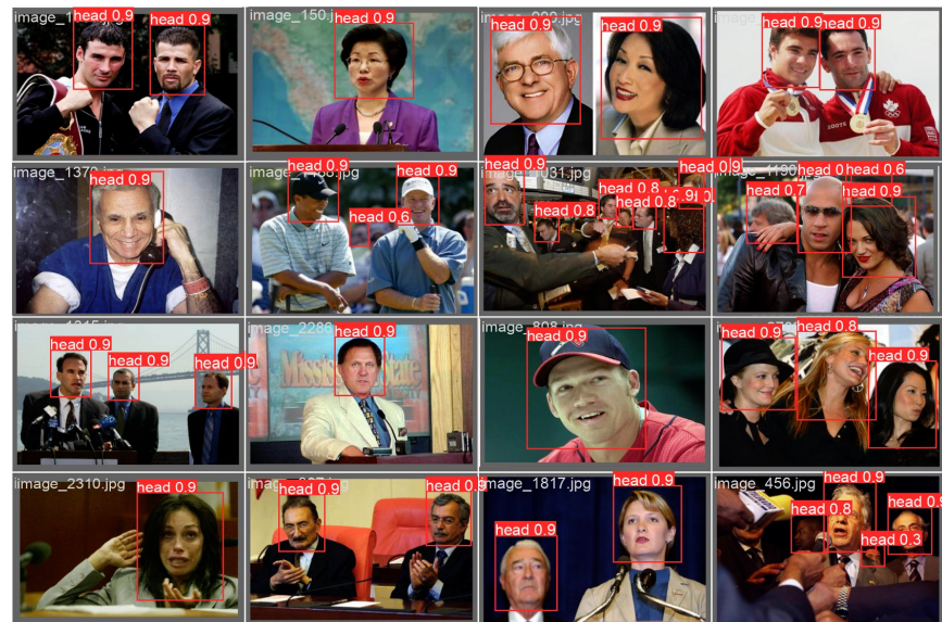
Figure 13. Head detection result samples of YOLOv8, where a red box denotes a detected head with its corresponding confidence level.
