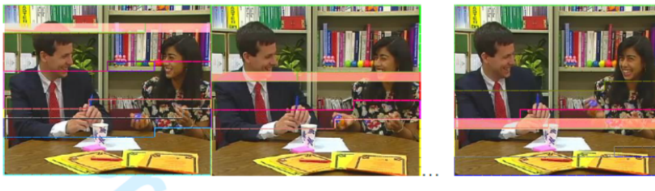
Figure 8. Example video frames from Paris, showing a cyclic Intra Refresh Line (IRL) and (optional) slices.
