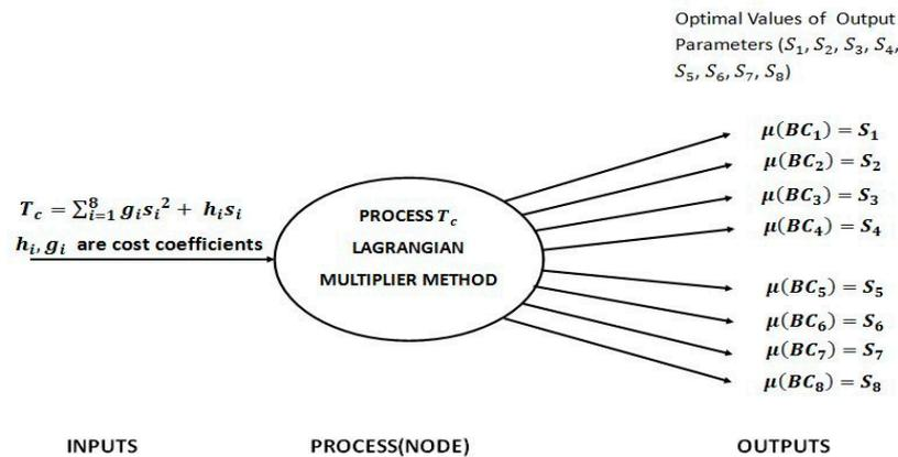
Figure 5. Data flow graph (DFG) of process  $T_c$  (Lagrangian multiplier method).
