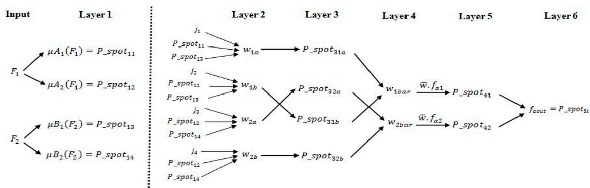
**Figure 10.** General architecture of a new modified ANFIS.
