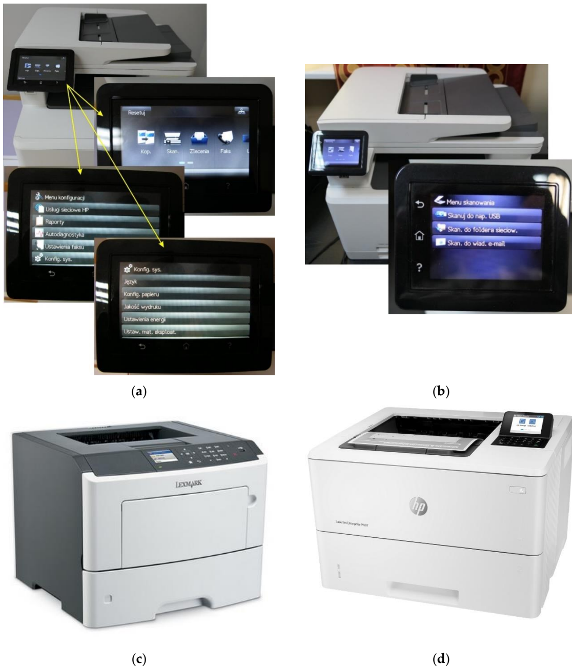
Figure 3. Four different laser printers used during tests of valuable emissions from displays: (a) Color Laser Jet Pro MFP M477fdn, (b) Color Laser Jet Pro MFP M277dw, (c) Lexmark MS610DE (a source: https://www.lexmark.com/pl_pl/printer/7693/Lexmark-MS610dn ), (d) HP 507 (a source: https://www8.hp.com/pl_pl/printers/product-details/19203858 ).
