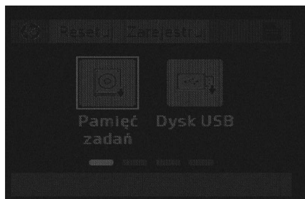
Figure 10. Image obtained on the basis of revealing emission measured on frequency f_0 = 1177 MHz ( BW = 100 MHz) for the source in form of printer display (Figure 3d).
