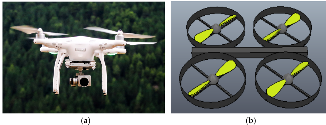
Figure 1. Example of quadrotor drones. The unmanned aerial vehicles are shown in both real-world and simulated environments. (a) DJI Phantom radio controlled quadrotor operating in a real environment; (b) Simulated quadrotor drone in V-REP used in the proposed domestic scenario.
