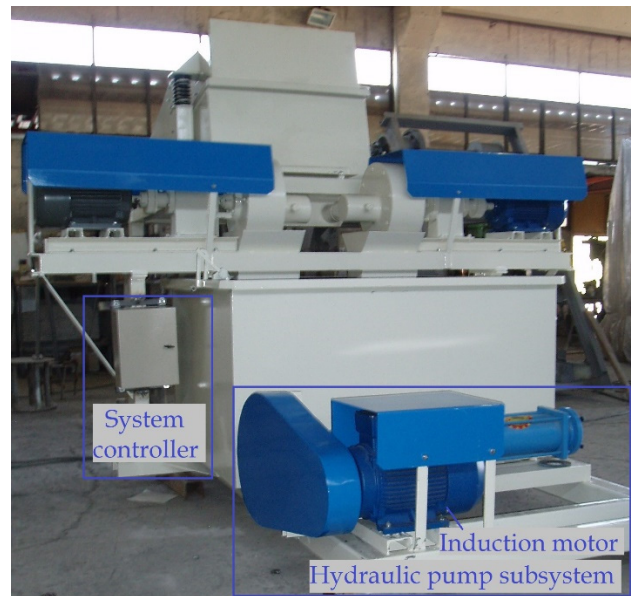
Figure 3. Lime milk storage and delivery machine.
