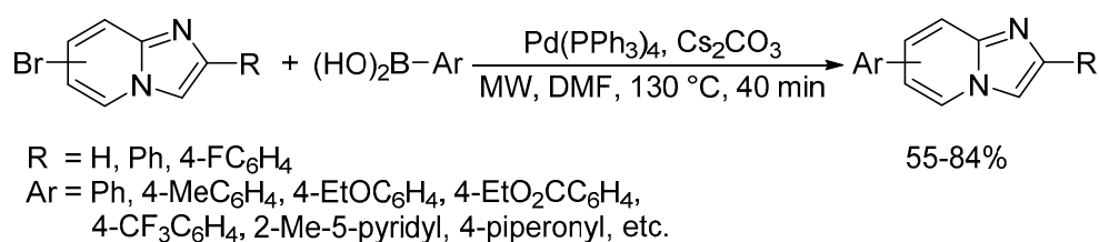
Scheme 32. Suzuki coupling reactions of bromoimidazo[1,2-a]pyridines and arylboronic acids.
