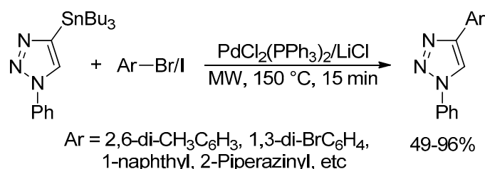
Scheme 39. PdCl 2 (PPh 3 ) 2 /LiCl mediated Stille coupling reactions.
