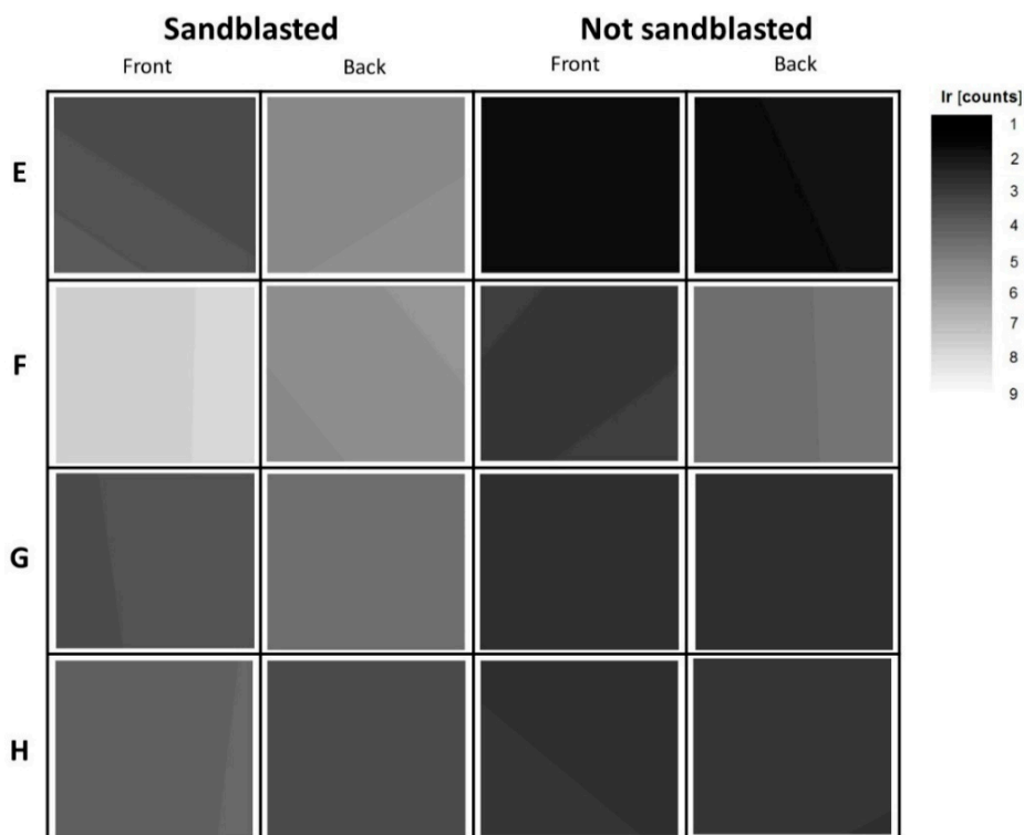
Figure 3. X-ray fluorescence (XRF) mapping of the IrO 2 samples in terms of iridium counts. Iridium counts range from 3 to 7. Darker shade means less iridium content.
