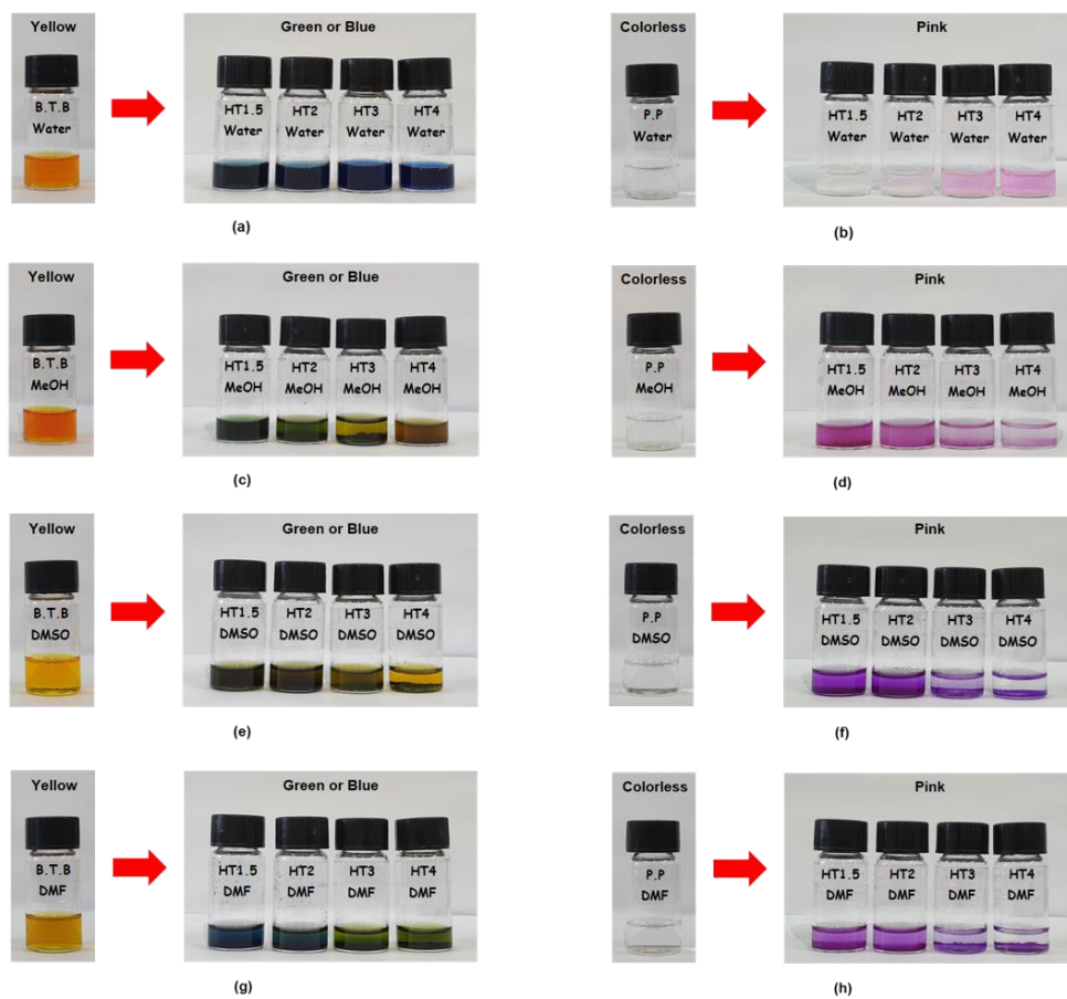
Figure S1. Hammett indicator method of prepared HTX catalyst ( X=1.5, 2, 3, and 4 ): (a) Bromothymol blue ( H_a=7.3 ) in water, (b) Phenolphthalein ( H_a=9.5 ) in water, (c) Bromothymol blue ( H_a=7.3 ) in MeOH, (d) Phenolphthalein ( H_a=9.5 ) in MeOH, (e) Bromothymol blue ( H_a=7.3 ) in DMSO, (f) Phenolphthalein ( H_a=9.5 ) in DMSO, (g) Bromothymol blue ( H_a=7.3 ) in DMF, (h) Phenolphthalein ( H_a=9.5 ) in DMF.
