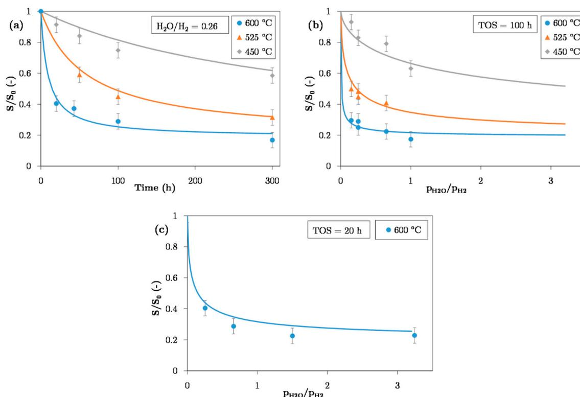
**Figure 7.** Comparison of experimental and modeled loss of metallic surface area (a) for 300 h hydrothermal aging at 450, 525 and 600 °C under  $\text{H}_2:\text{H}_2\text{O}$  atmosphere, with a  $\text{H}_2\text{O}$  to  $\text{H}_2$  ratio of 0.26; for several  $\text{H}_2\text{O}$  to  $\text{H}_2$  ratios (b) for 100 h at 450, 525 and 600 °C and (c) for 20 h at 600 °C.
