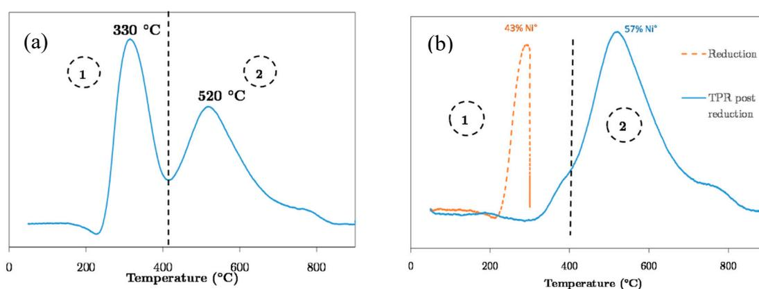
**Figure 1.** (a)  $\text{H}_2$ -TPR of the fresh commercial catalyst Ni/ $\text{Al}_2\text{O}_3$ ; (b) Activation procedure at 300 °C followed by a  $\text{H}_2$ -TPR from 50 until 900 °C.
