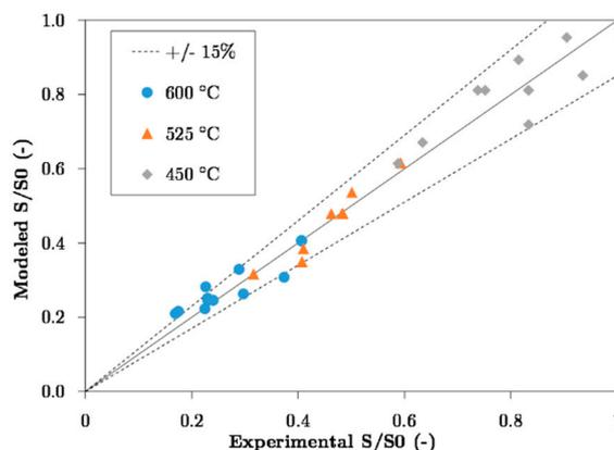
**Figure 8.** Parity plot of the experimental and modeled metallic surface area up to 300 h aging within 15% error at 450, 525 and 600 °C for a H<sub>2</sub>O:H<sub>2</sub> ratio ranging from 0 to 3.2.
