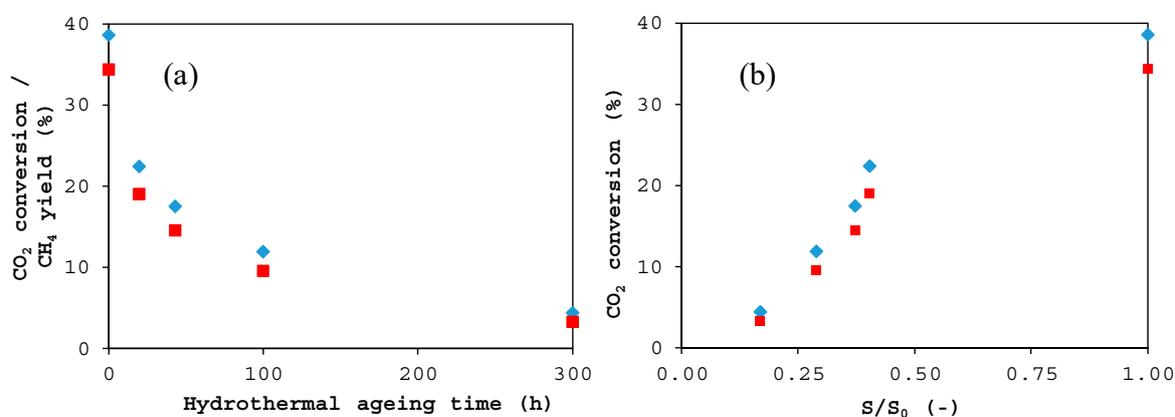
**Figure 2.** Catalyst activity measurements at 350 °C of fresh and post mortem samples aged at 600 °C in hydrothermal conditions ( $\text{H}_2:\text{H}_2\text{O} = 0.26$ ) as a function of hydrothermal ageing time (a) and relative metallic surface (b) ♦:  $\text{CO}_2$  conversion ■:  $\text{CH}_4$  yield.
