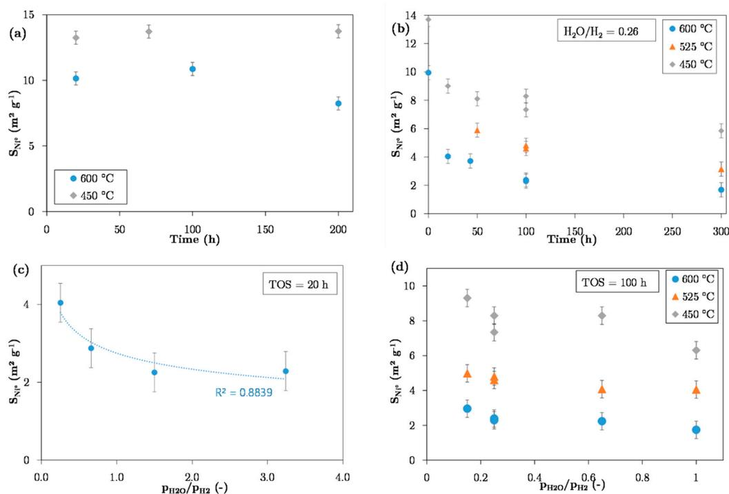
**Figure 3.** (a) Effect of temperature on metal particle sintering in reductive atmosphere H<sub>2</sub>:N<sub>2</sub>; (b) effect of temperature on metal particle sintering under H<sub>2</sub>:H<sub>2</sub>O atmosphere, with a H<sub>2</sub>O to H<sub>2</sub> ratio of 0.26; effect of H<sub>2</sub>O to H<sub>2</sub> ratio on metal particle sintering (c) for 20 h at 600 °C and (d) for 100 h at 450, 525 and 600 °C.
