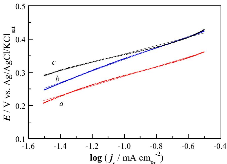
**Figure 6.** Tafel plots corresponding to the linear sweep voltammograms of Figure 5b. Methanol oxidation in 1.0 M methanol + 0.5 M H<sub>2</sub>SO<sub>4</sub> on the Pt(Ni)/C 3:1 (a) and 8:1 (b) catalysts, compared to that of Pt/C (c).
