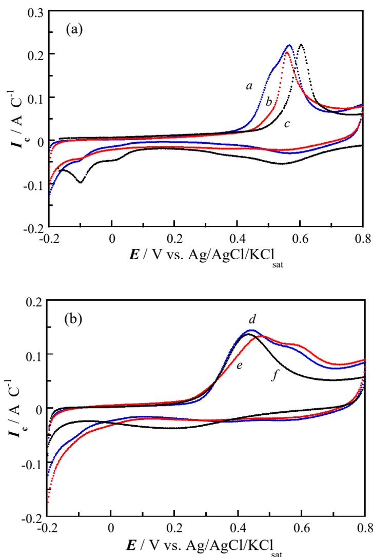
**Figure 4.** CO stripping experiments on the different catalysts in deaerated 0.5 M H<sub>2</sub>SO<sub>4</sub>. (a) Pt(Ni)/C 3:1 (curve *a*) and 8:1 (*b*), compared to Pt/C (*c*). (b) PtRu(Ni)/C 3:1 (curve *d*) and 8:1 (*e*), compared to commercial PtRu/C (*f*). Curves normalized to the CO stripping charge. Sweep rate 20 mV s<sup>-1</sup>.
