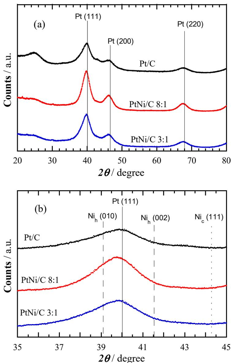
**Figure 2.** (a) XRD diffractograms of the catalysts studied, where that of Pt/C has been included for comparison. (b) Magnification of the XRD profiles shown in (a) in the Pt (111)  $2\theta$  region, including the diffraction angles of hexagonal and cubic Ni.
