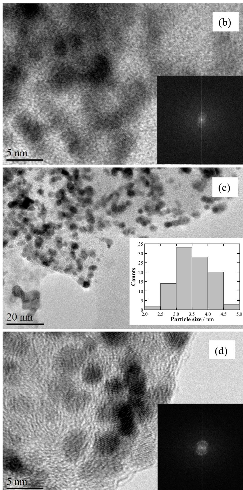
**Figure 3.** TEM pictures and size distribution of the nanoparticles of (a) Pt(Ni)/C 3:1 and (c) Pt(Ni)/C 8:1. The high resolution images of Pt(Ni)/C 3:1 and Pt(Ni)/C 8:1 are given in (b,d), respectively, together with the corresponding FFT pictures presented in the insets.
