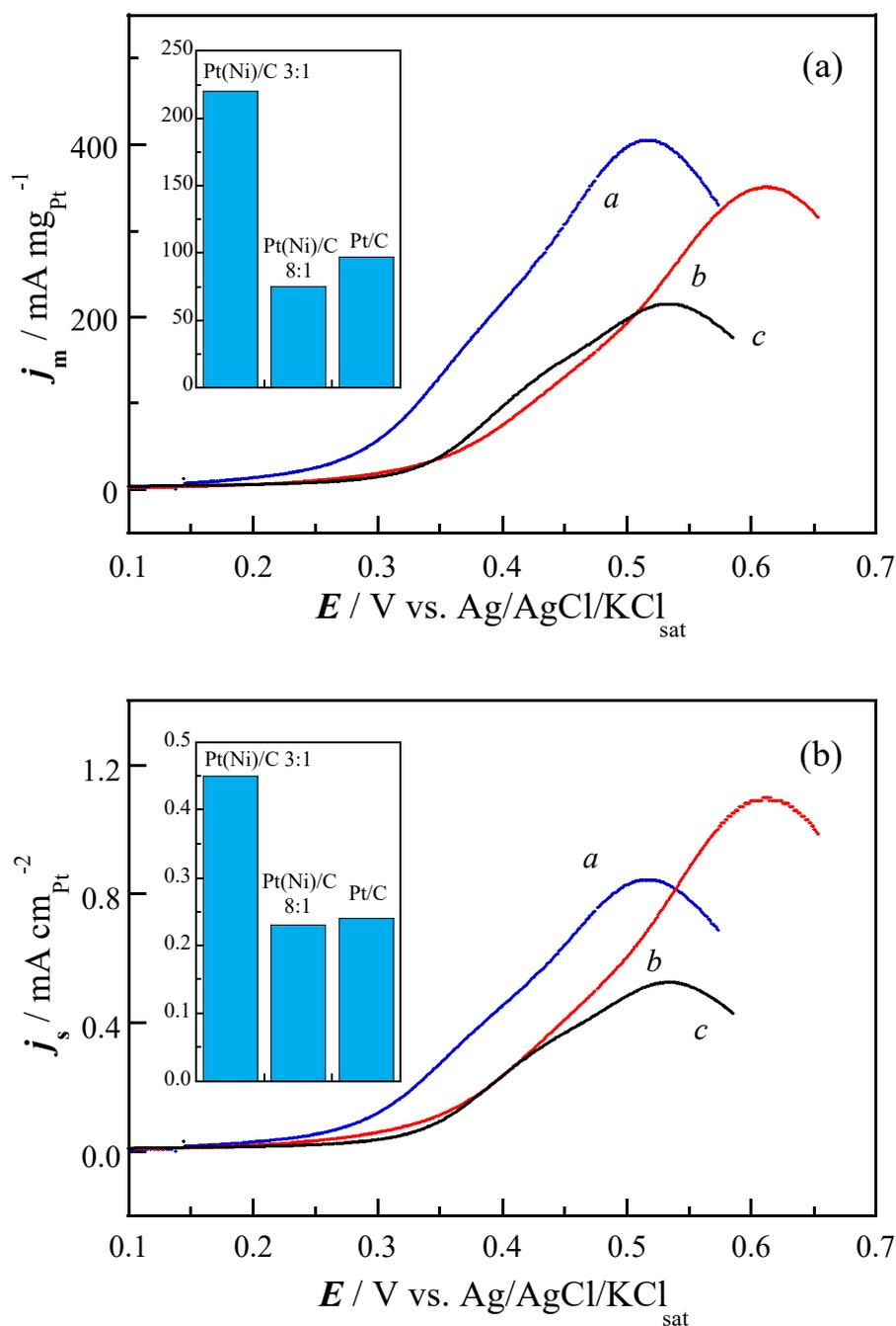
**Figure 5.** Linear sweep voltammograms obtained for the methanol oxidation in 1.0 M methanol +0.5 M H<sub>2</sub>SO<sub>4</sub> on the Pt(Ni)/C 3:1 (curves *a*) and 8:1 (curves *b*), compared to those of Pt/C (curves *c*), corresponding to (a) the mass activities  $j_m$  and to (b) the specific activities  $j_s$ . Sweep rate of 20 mV s<sup>-1</sup>. The  $j_m$  and  $j_s$  values at 0.4 V are given in the insets.
