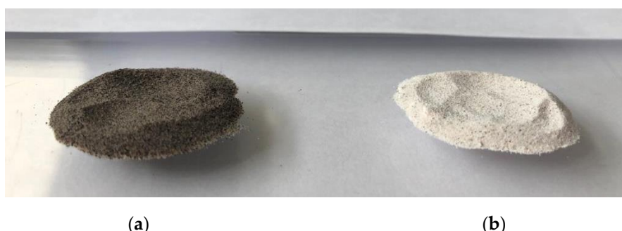
Figure A5. Coke deposition after 30 s of reaction time, at 500 °C in the CREC riser simulator: (a) \gamma -Al 2 O 3 , (b) 10% CaO- \gamma -Al 2 O 3 . Note: model compound: 2M4MP, S/B = 1.0.
