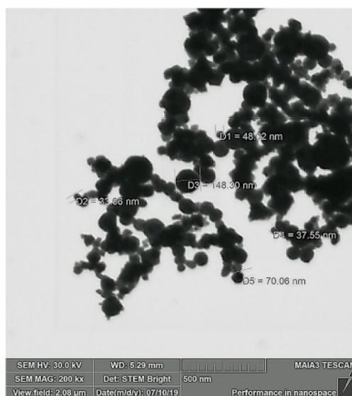
Figure 1. TEM micrograph of 1.0 M ethanolic suspension of commercial 25 nm zero valent iron nanoparticles (ZVI-NPs).
