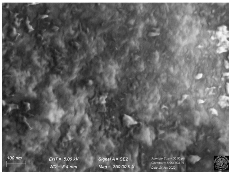
**Figure 5.** SEM of Cat1\* 0.25%Pd/Al<sub>2</sub>O<sub>3</sub> (250000 magnifications)
