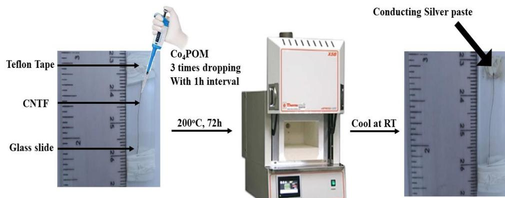
**Figure 6.** Schematic illustration of electrode fabrication by drop casting.
