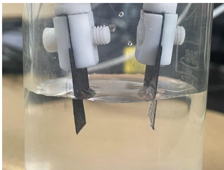
Figure S16 The equipment picture of alkaline OWS test in 1 M KOH solution.
