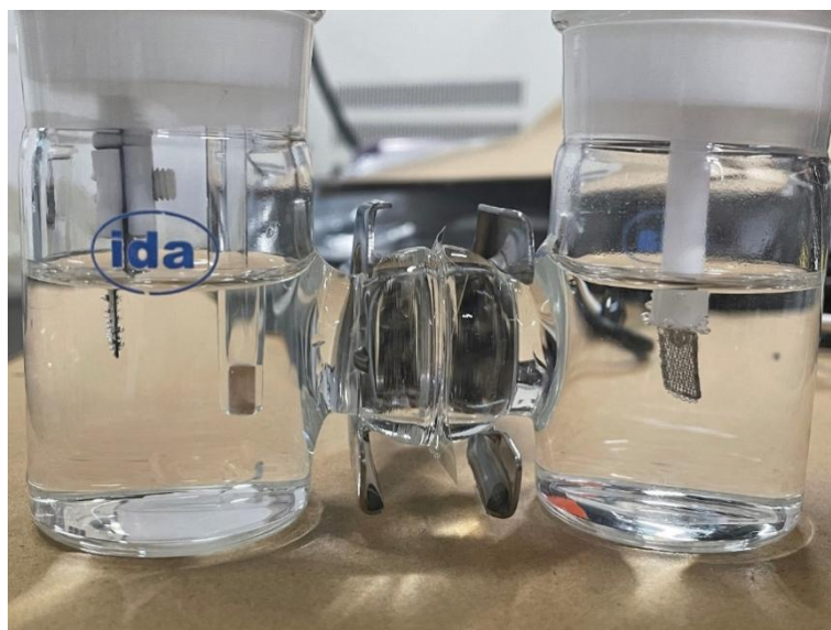
Figure S6 The equipment picture of alkaline HER test in 1 M KOH solution.
