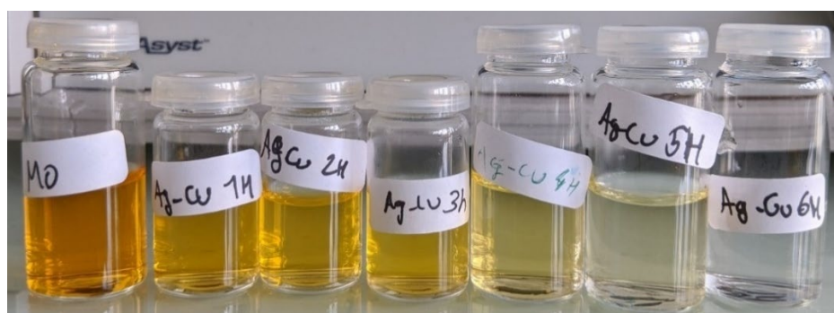
Figure 13. Colour of MO dye after 0 to 6 h of catalyst treatment in the presence of H_2O_2 .
