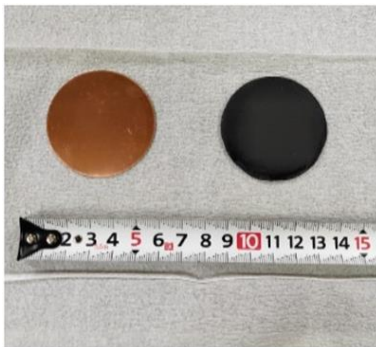
Figure 5. Photo of black body material prepared by this study and Cu solid disc before spraying black body spray.
