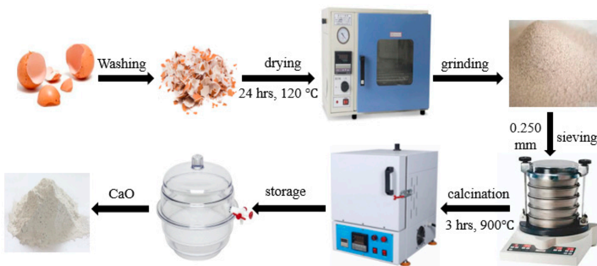
Figure 15. Schematic diagram of CaO synthesis.
