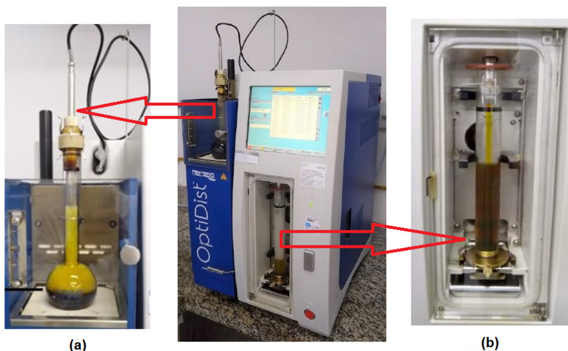
Figure 10. Equipment used for automatic distillation according to ASTM D86: (a) the reactor containing the atmospheric residue of the petroleum and catalyst; (b) glass measuring cylinders with 100 mL capacity to collect the distilled products.
