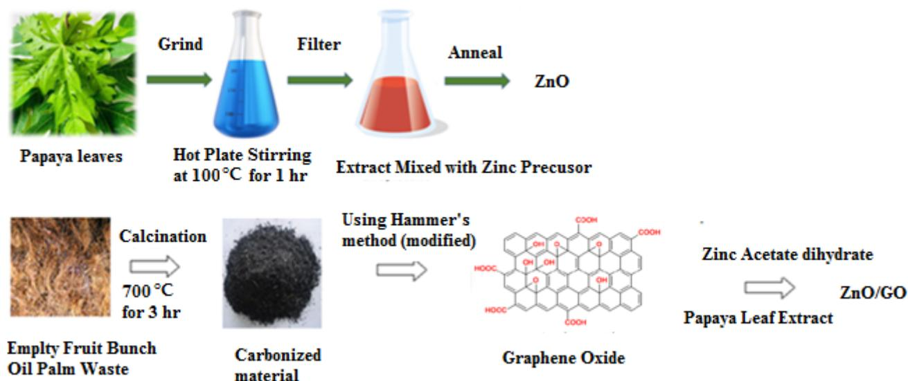
Figure 11. A systematic diagram showing the green synthesis method for ZnO and ZnO/GO.
