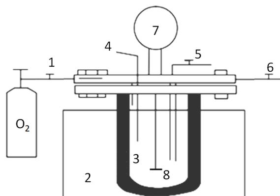
**Figure 8.** Diagram of wet oxidation reactor. 1—oxygen supply, 2—heating jacket, 3—oxidation reactor, 4—thermocouple, 5—discharge of gas, 6—bleeder valve, 7—pressure meter, and 8—stirrer.
