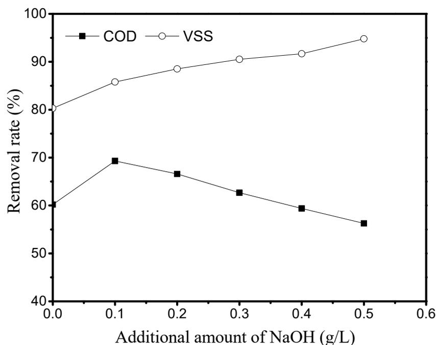
**Figure 1.** Effect of additional amount of NaOH (260 °C, 60 min, initial oxygen supply 1.0 MPa).
