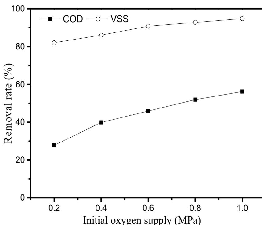
**Figure 4.** Effect of initial oxygen supply (260 °C, 60 min, NaOH 0.5 g·L<sup>-1</sup>).
