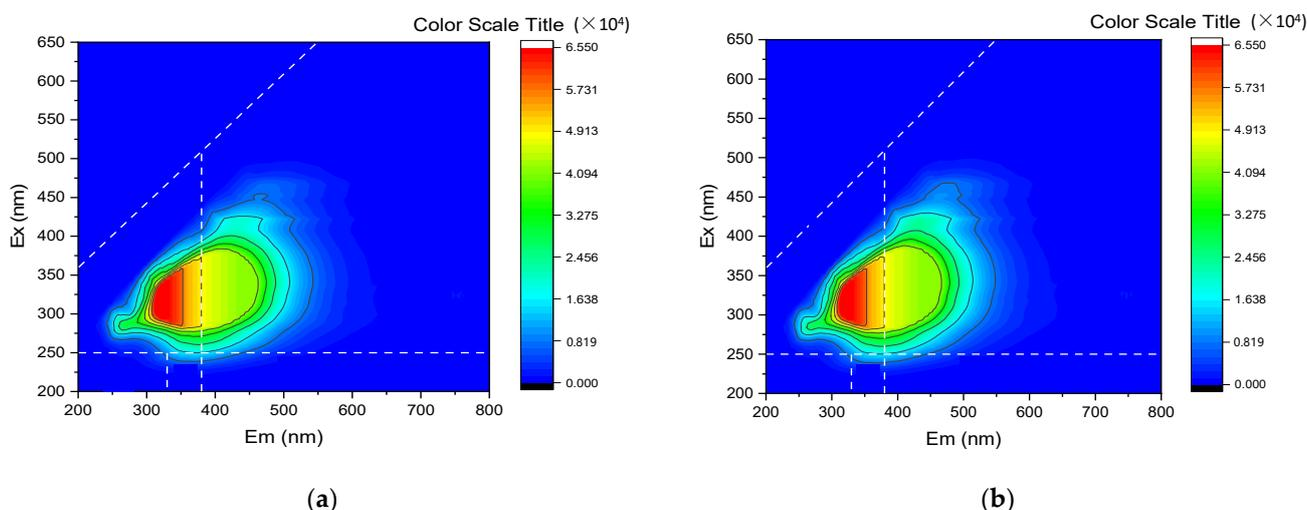
**Figure 5.** 3D Excitation-emission matrix spectra of wet oxidation liquid (a): without NaOH; (b): with NaOH.
