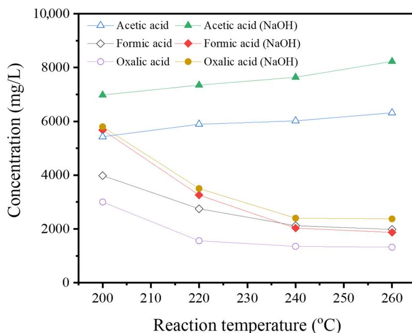
**Figure 6.** Concentration of carboxylic acids in wet oxidation liquid.
