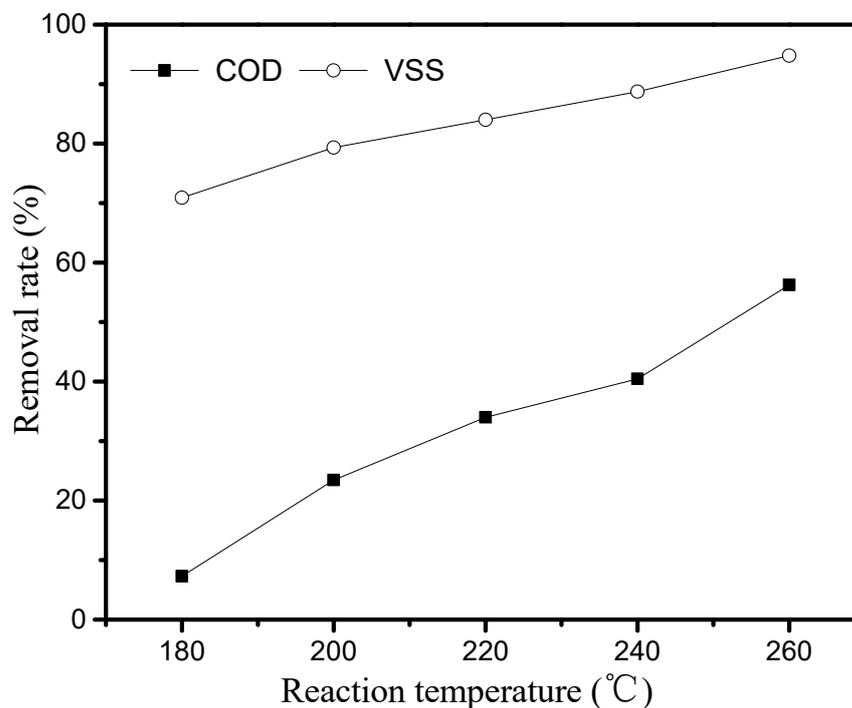
**Figure 2.** Effect of reaction temperature (60 min, NaOH 0.5 g·L<sup>-1</sup>, initial oxygen supply 1.0 MPa).
