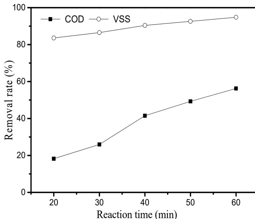
**Figure 3.** Effect of reaction time (260 °C, NaOH 0.5 g·L<sup>-1</sup>, initial oxygen supply 1.0 MPa).
