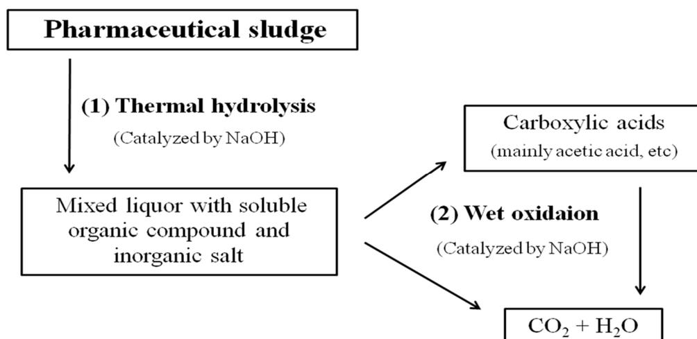
**Figure 7.** Diagram of the proposed degradation pathway.
