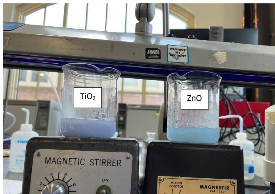
Figure S.7. Photograph of experimental tests showing the decolorization of 0.01 mM methylene blue solution in deionized water. Photocatalyst = 0.5 g/L. Light intensity = 3.2 \pm 1.3 mW/cm 2 .
