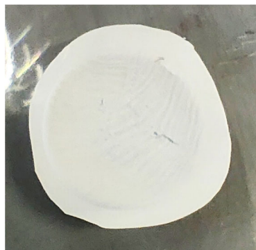
Figure 10. Picture of a membrane with physical damage after UP filtration.
