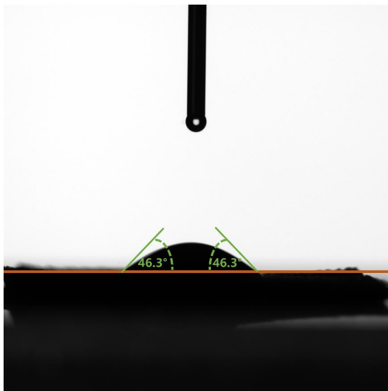
Fig. S6. NiFeP@FeOOH/NF contact angle test.
