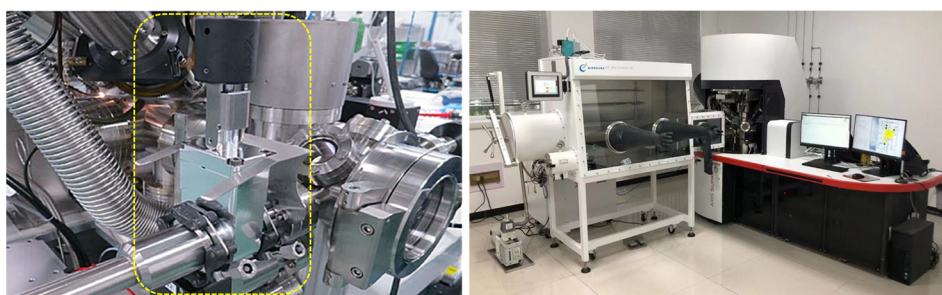
Figure 9. A sample transfer under vacuum or inert gas (left) from Kratos Analytical and a glovebox (right) connected to the instrument's pre-pumping chamber.
