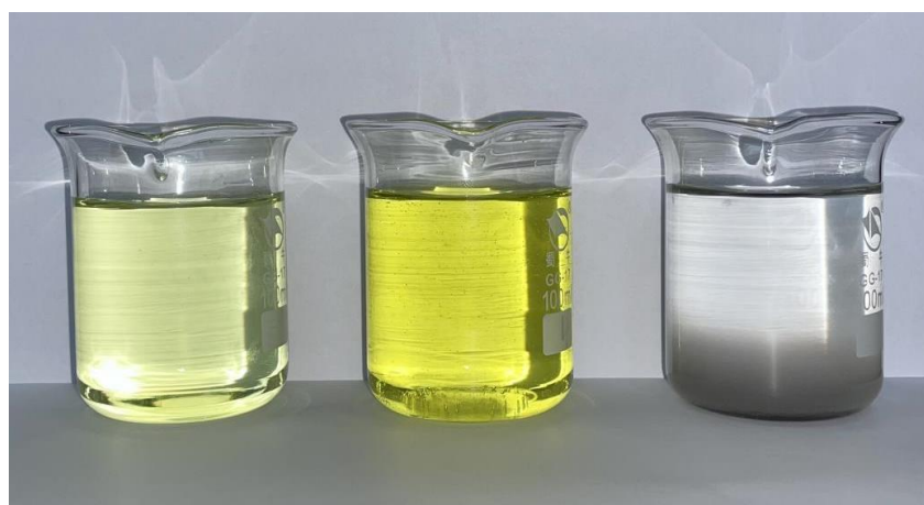
Figure S2. Left p-NP; Middle p-NP added to NaBH 4 ; Right After addition of catalyst reaction.
