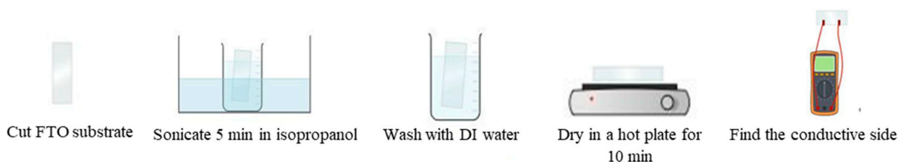
Figure 6. Scheme diagram for FTO glass pretreatment.
