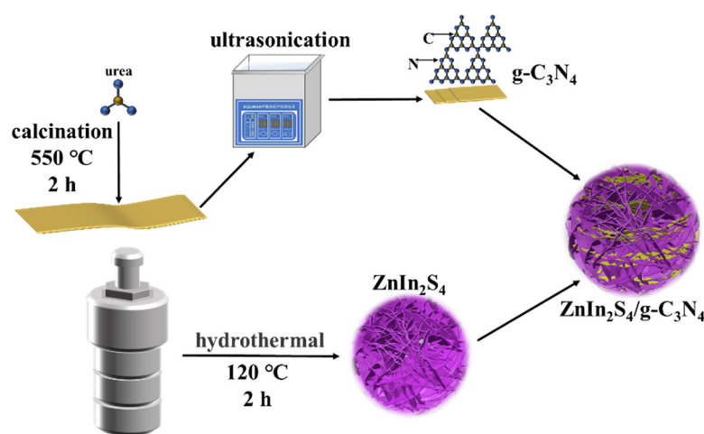
Scheme 1. The preparation process of \text{ZnIn}_2\text{S}_4/g\text{-C}_3\text{N}_4 .
