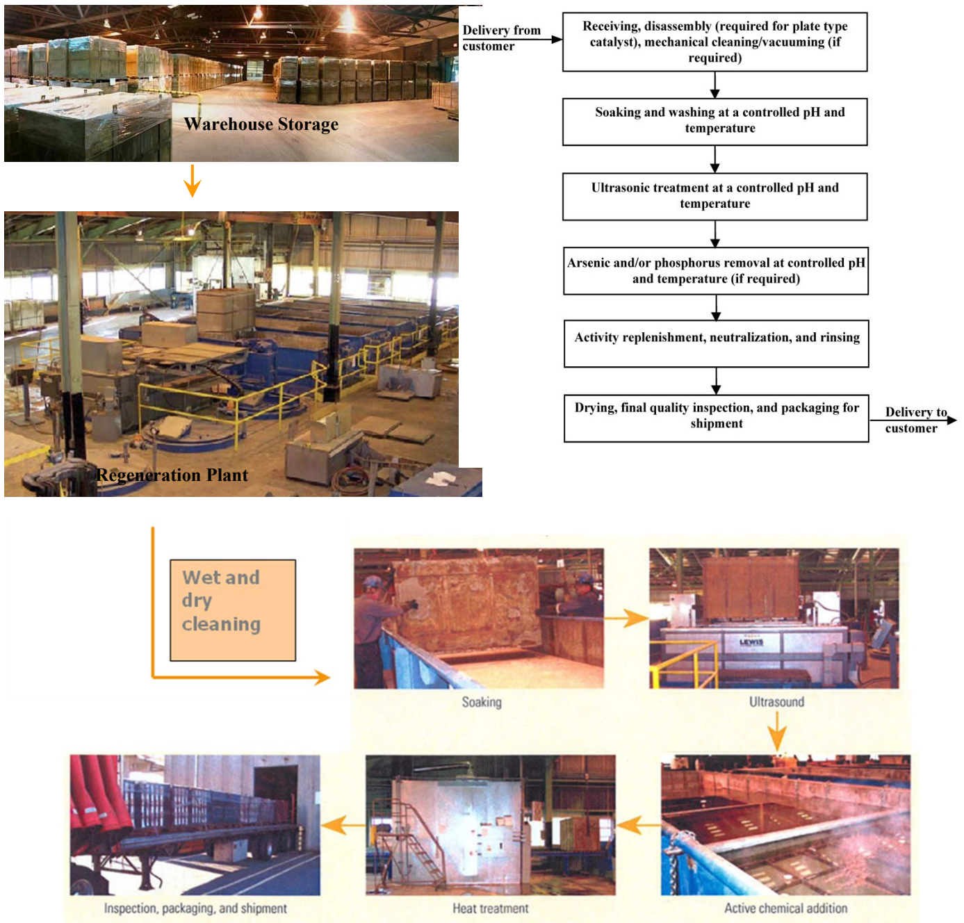
Figure 43. SCR-Tech catalyst regeneration process. Reproduced from [322,335–337]. Reproduced with permission of Electric Power and CoaLogix, Inc.
