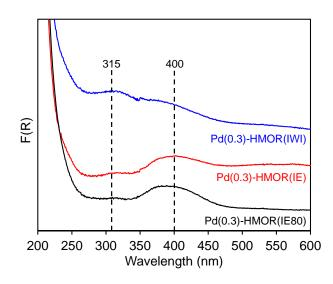
**Figure 2.** Diffuse Reflectance UV-Vis spectra of Pd(0.3)-HMOR catalysts prepared by different methods.
