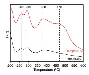
**Figure 8.** Diffuse Reflectance UV-Vis spectra of PdCe-HMOR catalysts containing 0.3 wt. % Pd and 2 wt. % Ce, introduced in different order.
