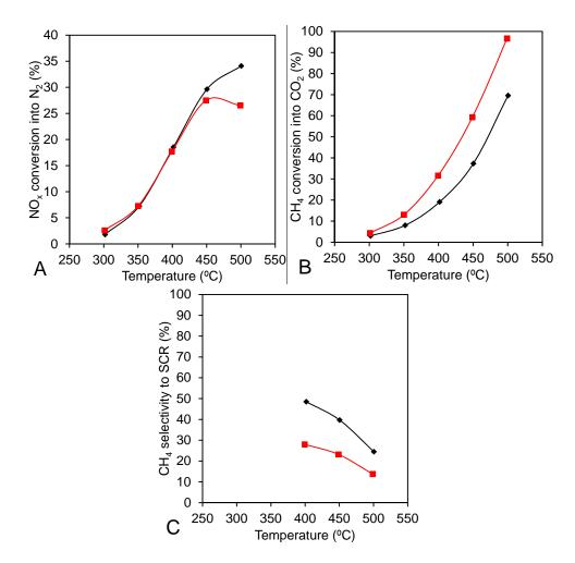
**Figure 9.** NO<sub>x</sub> conversion into N<sub>2</sub> (**A**); CH<sub>4</sub> conversion into CO<sub>2</sub> (**B**) and CH<sub>4</sub> selectivity to SCR reaction (**C**) over PdCe-HMOR catalysts containing 0.3 wt. % Pd and 2 wt. % Ce, introduced in different order. Conditions: 1000 ppm NO; 1000 ppm CH<sub>4</sub>, 7 vol % O<sub>2</sub>; and GHSV of 40000  $h^{-1}$ .
