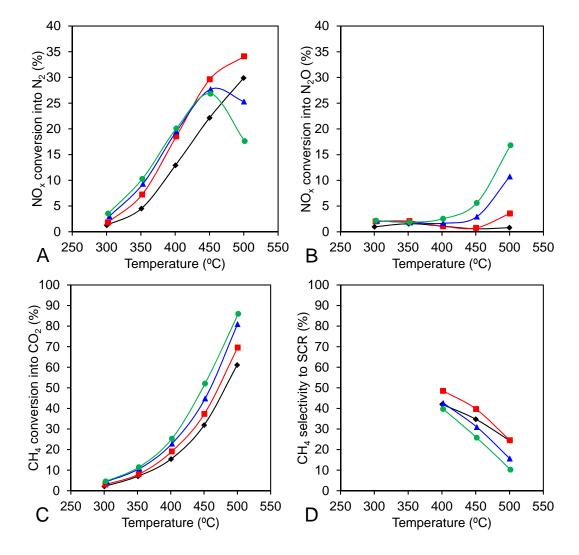
**Figure 6.** NO<sub>x</sub> conversion into N<sub>2</sub> (**A**) and into N<sub>2</sub>O (**B**); CH<sub>4</sub> conversion into CO<sub>2</sub> (**C**); and CH<sub>4</sub> selectivity to SCR reaction (**D**) over PdCe-HMOR containing 2 wt. % of Ce and different loadings of Pd with 1000 ppm NO, 1000 ppm CH4, 7 vol % O<sub>2</sub>, and GHSV of 40,000 h<sup>-1</sup>: Pd(0.15)Ce(2)-HMOR (•); Pd(0.3)Ce(2)-HMOR (•), Pd(0.5)Ce(2)-HMOR (•).
