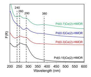
Figure 5. Diffuse Reflectance UV-Vis spectra of Pd(x)Ce(2)-HMOR catalysts.
