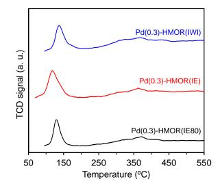
**Figure 1.** H<sub>2</sub>-TPR profiles of Pd(0.3)-HMOR catalysts prepared by different methods: ion-exchange at 80 °C (IE80), ion-exchange at room temperature (IE), and incipient wetness impregnation (IWI).
