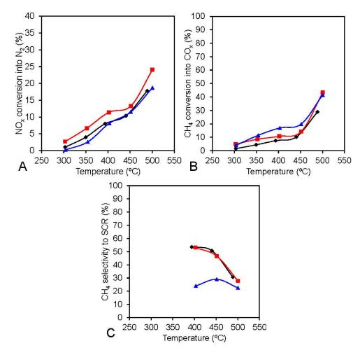
**Figure 3.** NO<sub>*x*</sub> conversion into N<sub>2</sub> (**A**); CH<sub>4</sub> conversion into CO<sub>*x*</sub> (**B**) and CH<sub>4</sub> selectivity to SCR (**C**) over Pd(0.3)-HMOR catalysts prepared by different methods: Pd(0.3)-HMOR(IE80) ( $\blacklozenge$ ); Pd(0.3)-HMOR(IE) ( $\blacksquare$ ); and Pd(0.3)-HMOR(IWI) ( $\blacktriangle$ ). Conditions: 1000 ppm NO, 1000 ppm CH<sub>4</sub>, 7 vol % O<sub>2</sub>, and GHSV of 40000 h<sup>-1</sup>.
