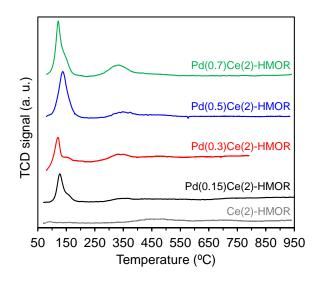
Figure 4. H<sub>2</sub>-TPR profiles of Pd(x)Ce(2)-HMOR catalysts.
