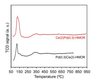
**Figure 7.** H<sub>2</sub>-TPR profiles of PdCe-HMOR catalysts containing 0.3 wt. % Pd and 2 wt. % Ce, introduced in different orders.
