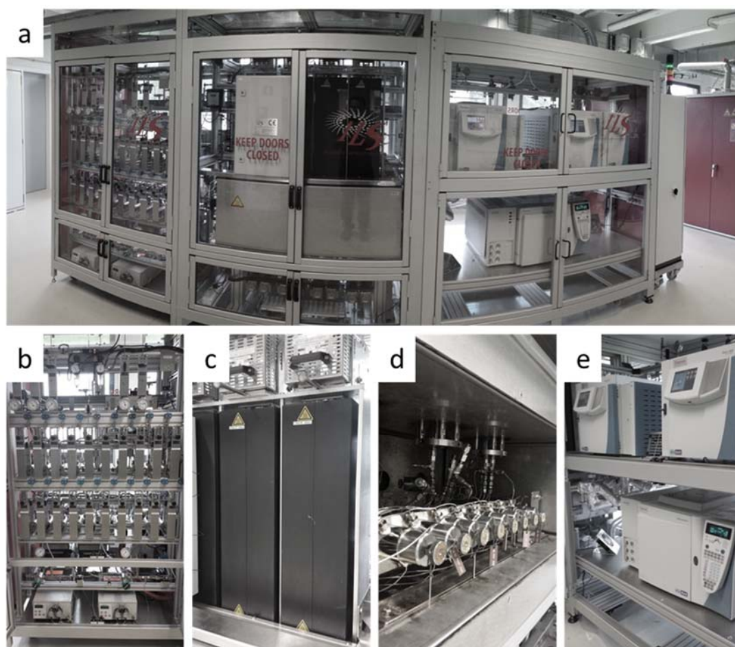
Figure 3. HTK-S set-up pictures: (a) front view; (b) gas (top) and liquid (bottom) feed section; (c) reactor heating blocks; (d) heated gas and liquid sampling section; and (e) analysis section.
