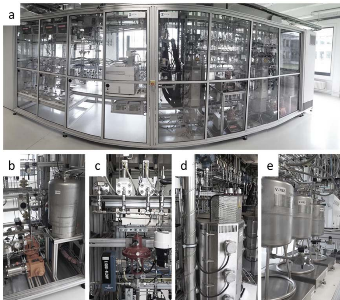
Figure 5. HTK-MI set-up pictures: (a) front view; (b) liquid pump section; (c) gas ( top ) and liquid ( bottom ) feed section; (d) reactor blocks; and (e) liquid waste collection.
