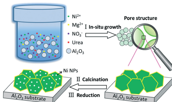
Figure 1. Schematic synthesis route of the catalysts from HTLc precursors grown in situ on an alumina substrate. Reproduced from [25] with permission of The Royal Society of Chemistry. Copyright 2014.
