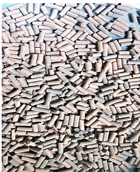
Figure 9. A photograph of prepared catalyst pellets.
