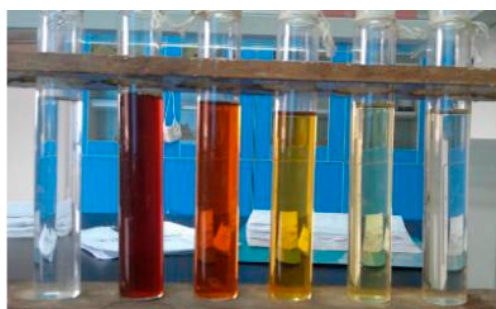
Figure 10. Effluent of catalytic-biological treatment portion (at 90th day). (Left to right: pure water/initial water/CBR-1/CBR-2/BAF-1/BAF-2).
