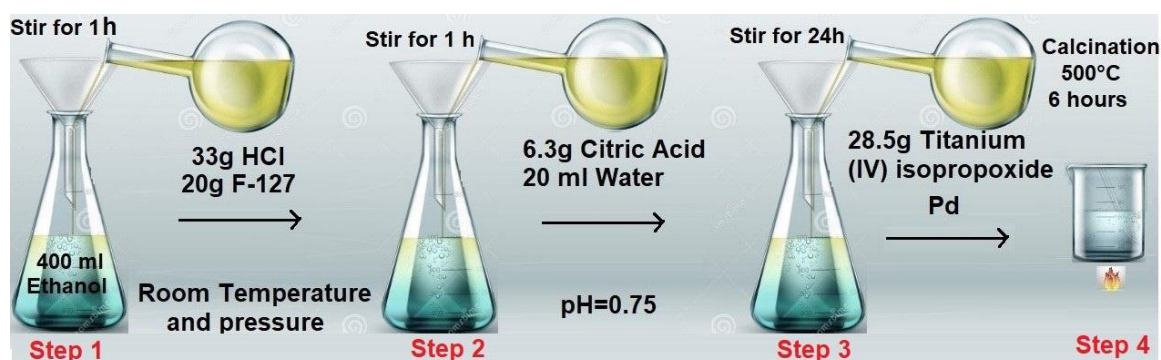
Figure 14. Photocatalyst preparation process describing the four steps considered for Pd-doped mesoporous.
