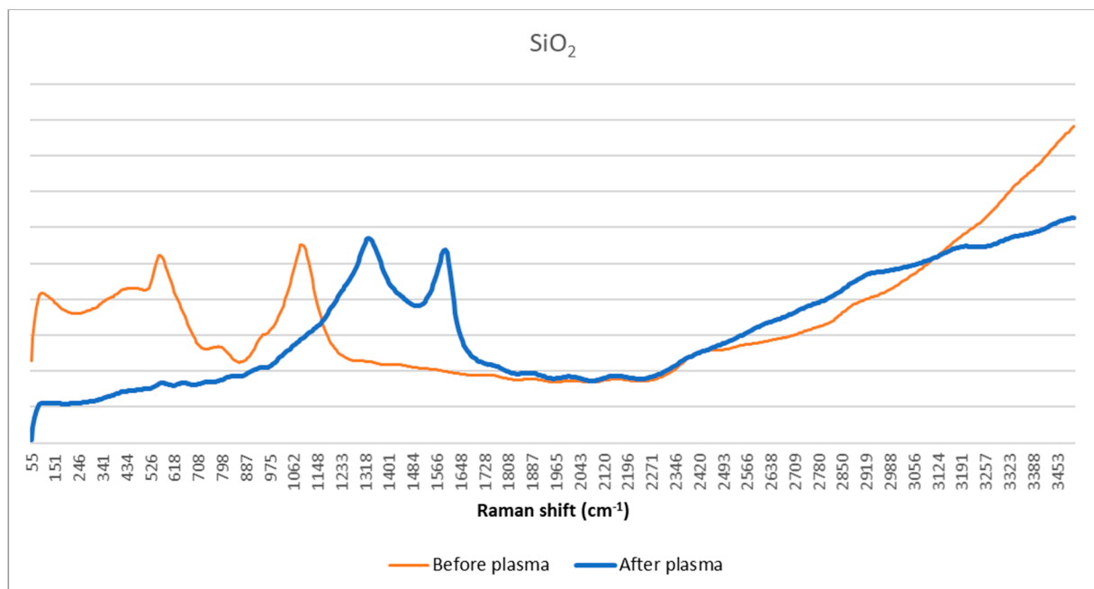
Figure S.16: Raman spectrum for SiO 2 , before and after plasma exposure.
